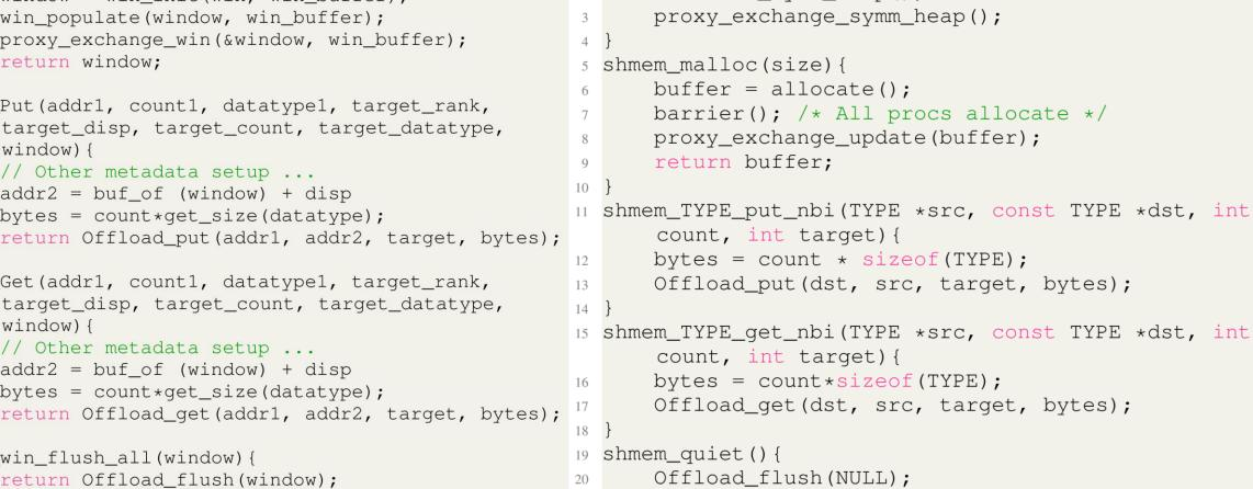
Proxy\_exchange in shmem\_malloc() there to "show" DPUs are aware of the usage of space in the symmetric heap.
