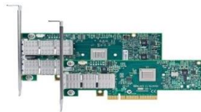
High Performance Interconnects - InfiniBand <1usec latency, >100Gbps Bandwidth
