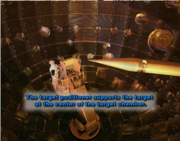
The target positioner supports the target at the center of the target chamber.
